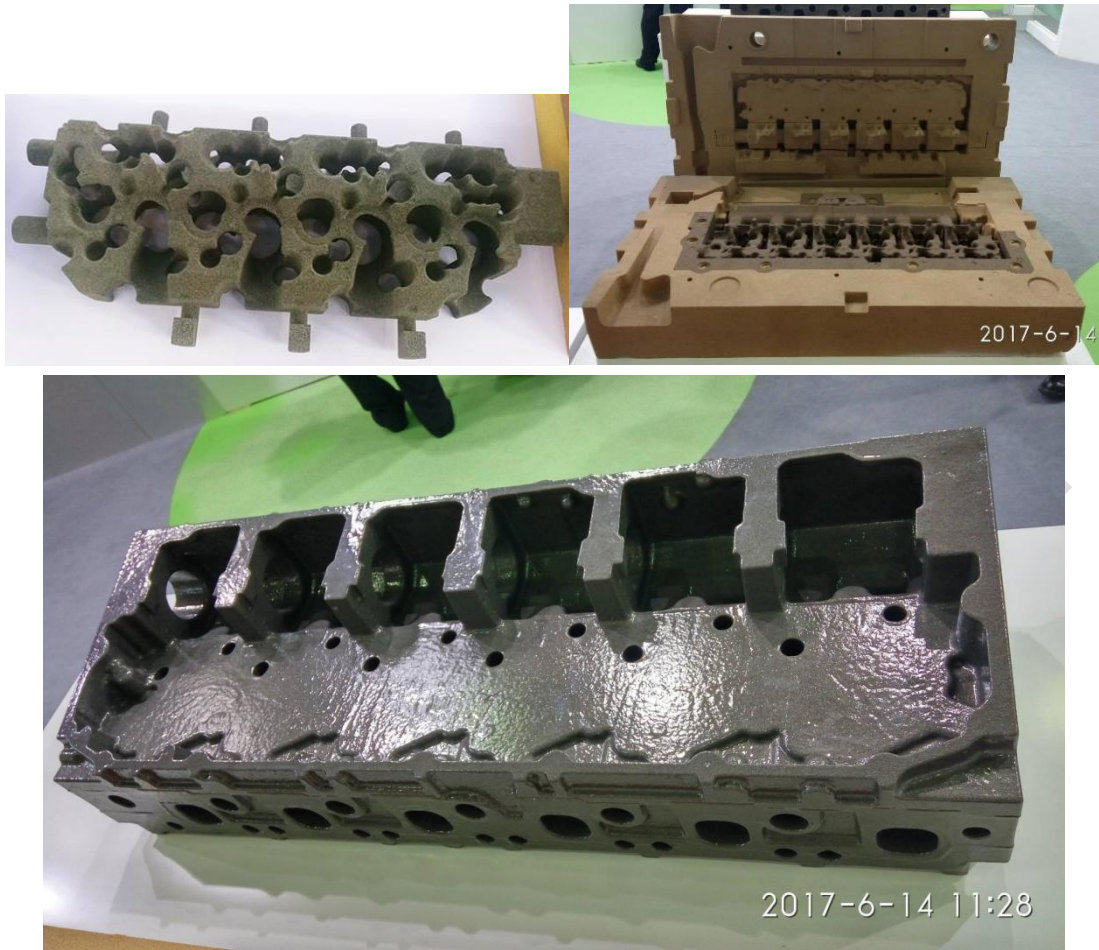
Fig. 6 Cylinder head, cylinder block, water jacket core and casting produced by Kailin Ceramic Sand cold-box process
