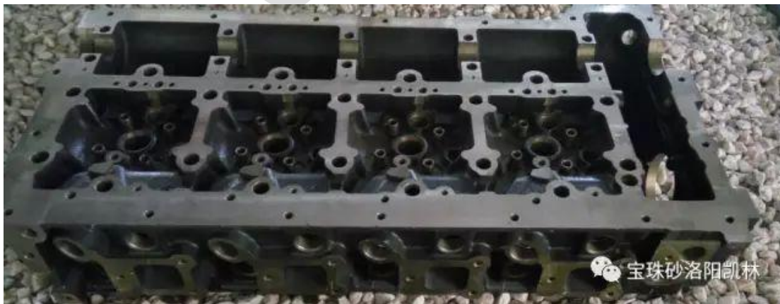
Fig. 5 Cylinder block and castings produced by Kailin Ceramic Sand cold-box process
